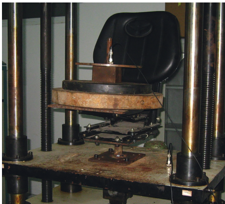
FIGURE 8: Site map of stiffness and damping test rig for the driver seat.
